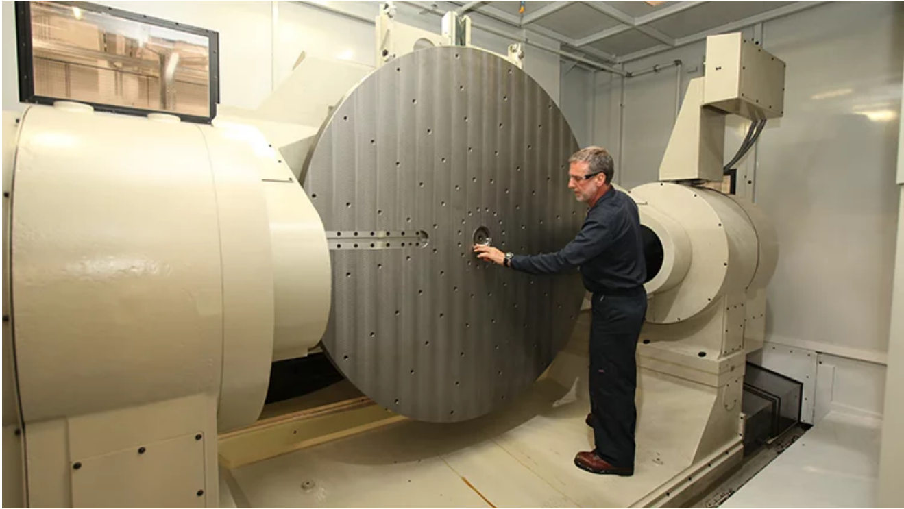
Mitsui Seiki's Wayne Wentworth stands in the work area of a five-axis Mitsui Seiki trunnion machining center. The table was custom engineered to accommodate a 78" (198-cm) diameter part.
